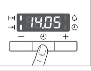
The function indicators Cook time  $\bowtie$  and End time  $\rightrightarrows$  light up and the current time is shown in the display. In this case 12:05.
